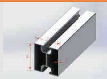
Beam Section: 80*70mm Material: AL6005-T5 Thickness of anodized films: \geq 12\mu\text{m}
