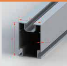
Rail Cross Profile 90*60mm Material: AL6005-T5 Thickness of anodized films: \geq 12\mu\text{m}
