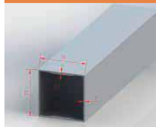
Column Cross Profile: 70*70mm Material: AL6005-T5 Thickness of anodized films: \geq 12\mu\text{m}
