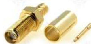
RSMA6421A1-3GT50G-8U-50 (RG-8U) RSMA6411A1-3GT50G-58U-50 (RG-58U) Conector Hembra, Crimp Tipo SMA (Pol. Invertida), 50 Ohm. Cable: RG-8U, RG-58U
