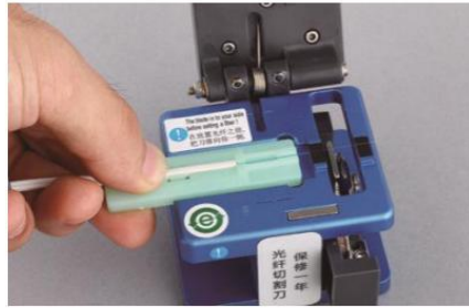
8.Press the cable into the groove and keep the fiber slightly bending
