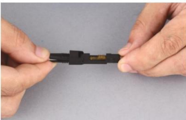
10.Close the gland for fixing drop cable
